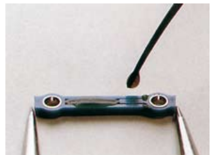
9 Block out the groove underneath the bar with wax before casting or further preparation.
