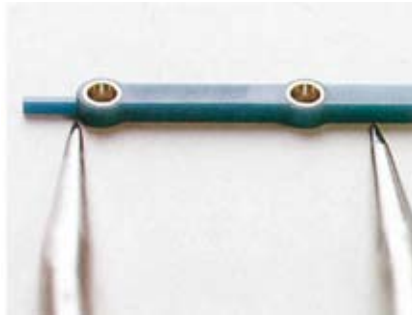
2 Place the bar at the tips of the dividers. Ensure that the width is not altered.
