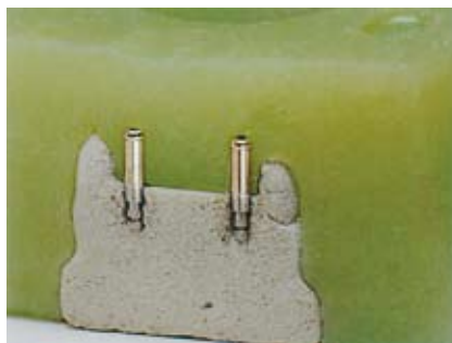
37 To ensure the retention screw is surrounded bubble-free with investment, cover it with investment before filling the duplicate mould.
