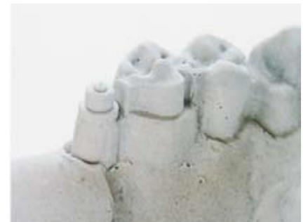
22 Duplicate according to instructions. The duplicating aid is clearly defined on the investment model after removal of the duplicating material.
