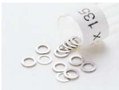
72 If the height of the plastic spacers has been altered due to incorrect preparation or polishing of the spacers, the spacer No. 135 or No. 235 for regulating the snap point can be inserted to restore the original snap point of the patrix.
