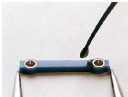
8 Wax the bar together at the junction.
