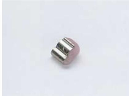
**9** Wax out the inside and underside of the matrix and sandblast the adhesive surface of the matrix and CrCo framework with aluminium oxide (250 µm).
