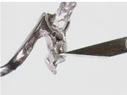
**14** Remove any excess adhesive after the DuroBond has hardened.
